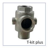
Stainless steel 5-ways fitting with inner non-return valve. Ideal for systems with hydropneumatic tank, with 2 inlets for pressure gauge and sensor element (transducer, pressure switch, ...).
