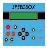
Control panel includes LCD screen, warning leds, push-buttons, START-STOP, AUTOMATIC and configuration system.
