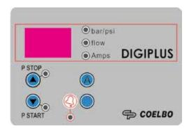
Control panel includes 3 digits display, warning leds, push-buttons and configuration system.
