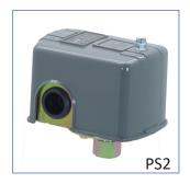
PS2 is the traditional mechanical pressure switch for pumps control up to 1,5 kW (2HP), single-phase power supply 110 $\div$ 230 V, protection degree IP20 and female hydraulic connection G1/4".
