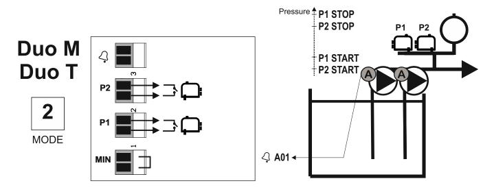
15.2.4. System of 2 pumps. Start/stop in sequence (one after one) with pressure switches and dry-run protection through a minimum level float switch. Redundant dry-run protection by instantaneous power consumption reading.
