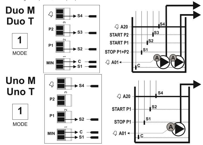
(\*) C is the common terminal for the electronic probes. It can be connected in anyone of the connectors. **15.1.5.** Drainage with float switches, 1 or 2 pumps. Connections on the HUB board. **Mode 2**.
