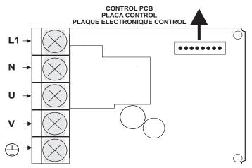
7.2.2.4 Power electronic circuit for 3-phase models.
