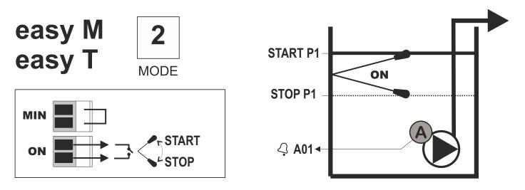
**15.1.2.** Start/stop by float switch and dry-run protection also by float switch. Redundant dry-run protection by instantaneous power reading. The connections will be carried out on the control board. **Mode 2.**
