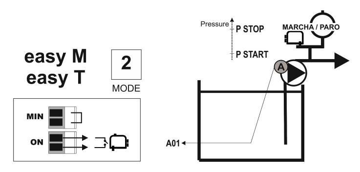
**15.2.2.** Start/stop by pressure switch and minimum level protection by float switch. Redundant dry-run protection by instantaneous power consumption reading. **Operation mode 2.**
