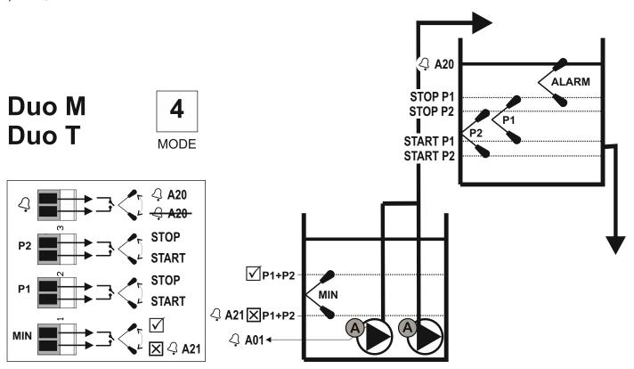
15.4.3. Start and stop managed by float switch. Float switch to activate/disable the pump in case of minimum liquid level on the well or cistern.
