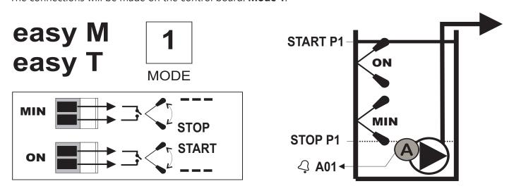
15.1.4. Drainage with probes, 1 or 2 pumps. Connetions in the HUB electronic board. Mode 1.
