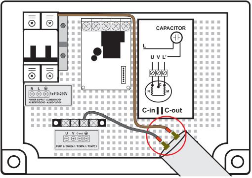
D1.2. Single-phase pump with capacitor and with HUB electronic board.
