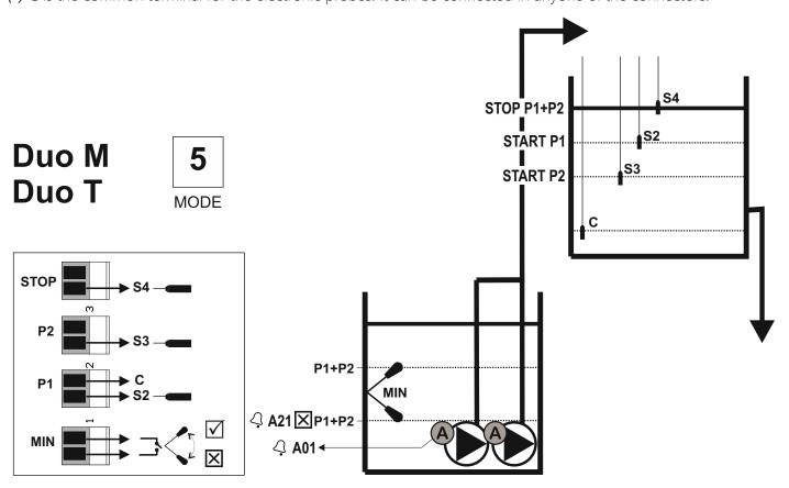
15.4.2. Start and stop managed by float switches. Float switch to activate/disable the pump in case of minimum liquid level on the well or cistern.
