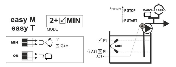
15.2.3. System of 2 pumps. Start/stop in sequence (one after one) with pressure switches and dry-run protection by instantaneous power consumption reading.
