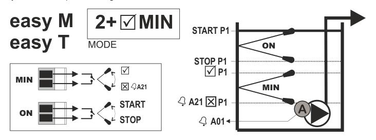
**15.1.3.** For narrow wells. Start and stop float switches. The connections will be made on the control board. **Mode 1**.
