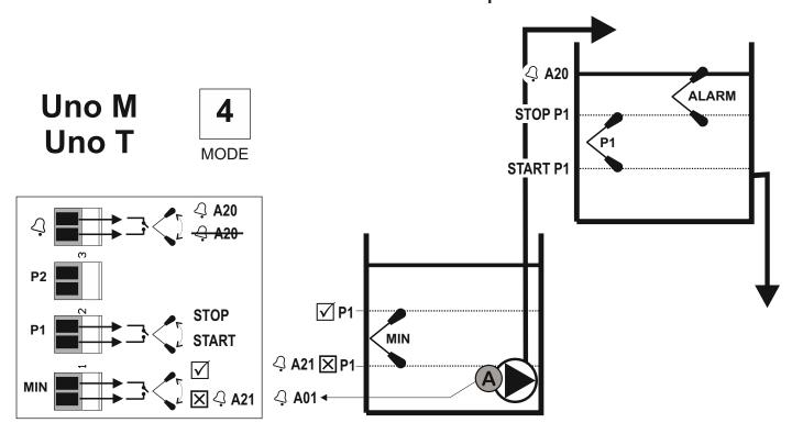
In case of 2 pump systems, they operate in **duty-assist** mode (one after one with alternated starting sequence).
