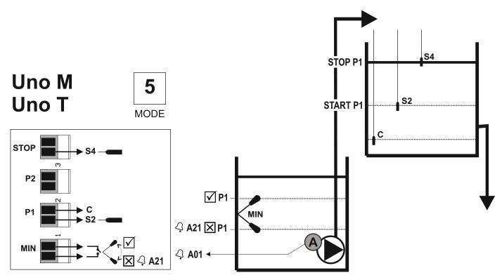
(\*) C is the common terminal for the electronic probes. It can be connected in anyone of the connectors.
